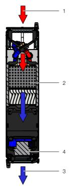
Fig. 2: Air routing on the LCP Inline DX - top view
