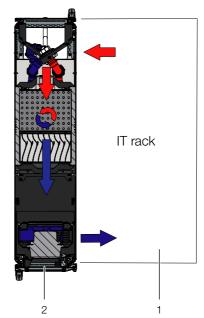
Fig. 4: Air routing with a bayed server enclosure – top view
