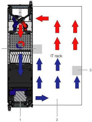
Fig. 16: Placement of foam strips for devices with sideways air throughput (top view) – LCP Rack DX
