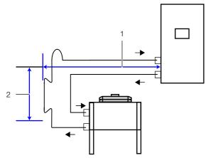
Fig. 12: Relative positioning condenser below the LCP DX
