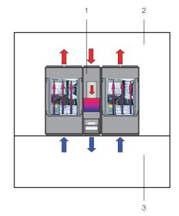
Fig. 14: Installation room with cold aisle containment
