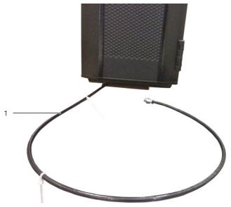
Fig. 22: Condensate discharge
