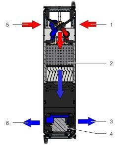
Air routing on the LCP Rack DX - top view Fig. 1:
