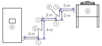
Fig. 21: Simplified representation of connection lines
